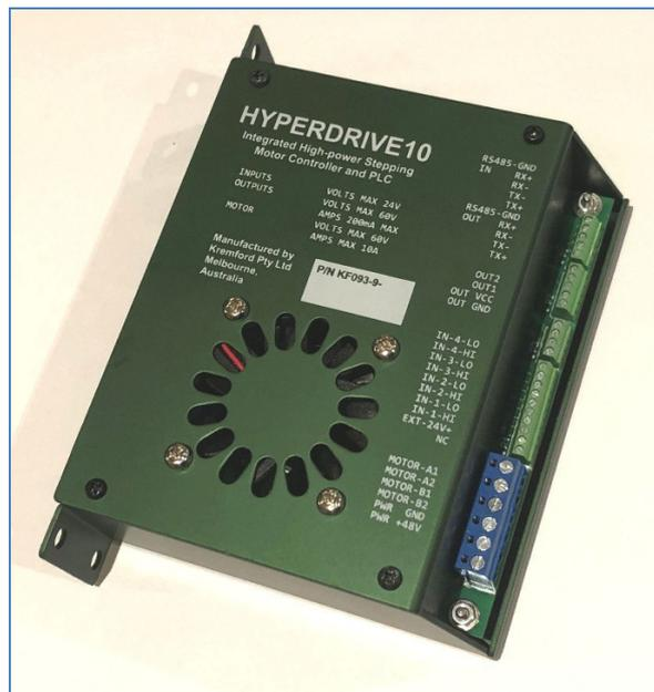
Figure 1. The Hyperdrive10 High Power Stepper Controller
