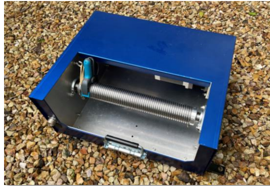
1. Customised electronically-controlled winch
